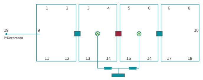
One 22kw surface aerator (colored red) with actual energy consumption of 19.42 kWh, was turned off and was replaced by 2 of Mapal's FFBA units connected to 12.5kw blower with actual energy consumption of 11.01kWh.
